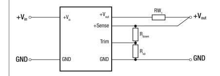
The output voltage can be adjusted via the trim and sense functions.
